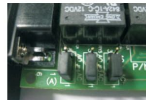
Fig. 6 Jumper setting for ACTIVE CLOSE
