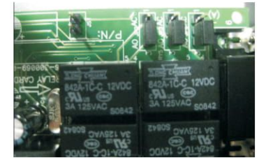
Fig. 5 AO and AC silk printings indicates each 3-pin connector status
