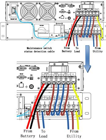
Connect power cables as above figure, and connect status signal cable between UPS and maintenance bypass if needed.
